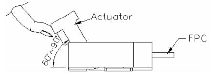
• The actuator opens by rotating it in the direction OPPOSITE to the direction of the insertion of the FPC. DO NOT attempt to open it from the same side as the insertion of the FPC.
